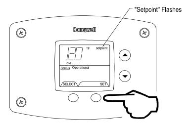
Step 3: To raise the temperature setpoint, press the "Temperature Up" button until the desired temperature is shown on the water heater display.
